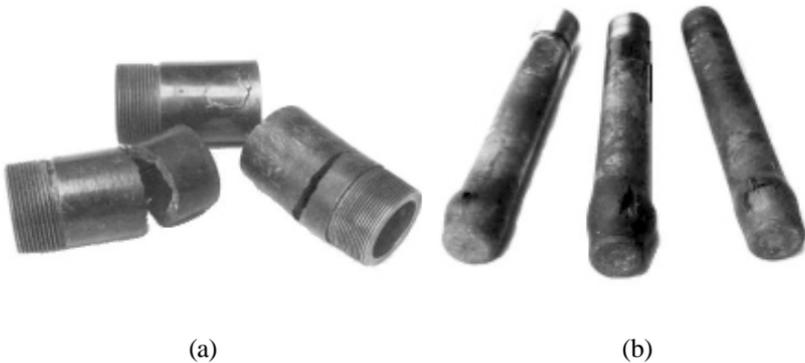
**Figure 3.40.** (a) Stellite Tuttle cold-cone sealed autoclaves and (b) stainless steel acid digestion bombs which ruptured at high pressure.
