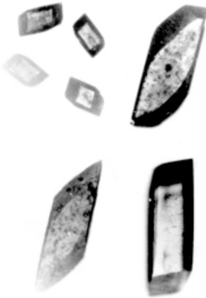
**Figure 7.67.** Photographs of  $\text{NaHZn}(\text{P}_2\text{O}_7)$  crystals (magnification  $\times 30$ ).<sup>[301]</sup>
