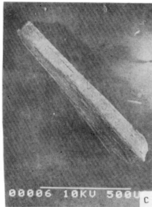
**Figure 7.81.** Photographs of  $\text{NH}_4\text{Zr}_2\text{V}_3\text{O}_{12}$  crystals obtained under hydrothermal conditions.<sup>[324]</sup>
