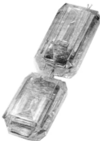
**Figure 7.27.** Two crystals resulting from one run still mounted on the silver seed holder and the baffle.<sup>[133]</sup>
