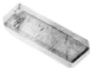
**Figure 8.29.** Sphalerite crystals grown under hydrothermal conditions.<sup>[99]</sup>
