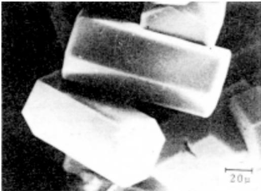
**Figure 7.32.** Hexagonal prism shaped crystals grown from 0.1 N NaOH solution.<sup>[162]</sup>
