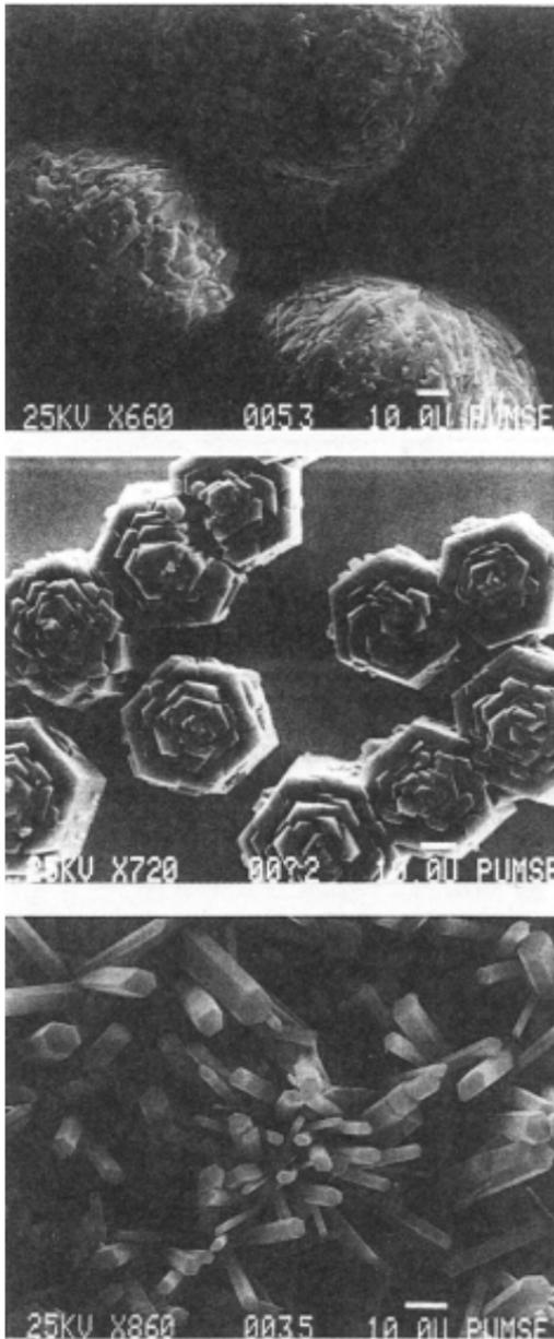
**Figure 6.37.** SEM pictures show that the AlPO<sub>4</sub>-5 crystals grow with their c-axes oriented similar to the gold surface.<sup>[124]</sup>
