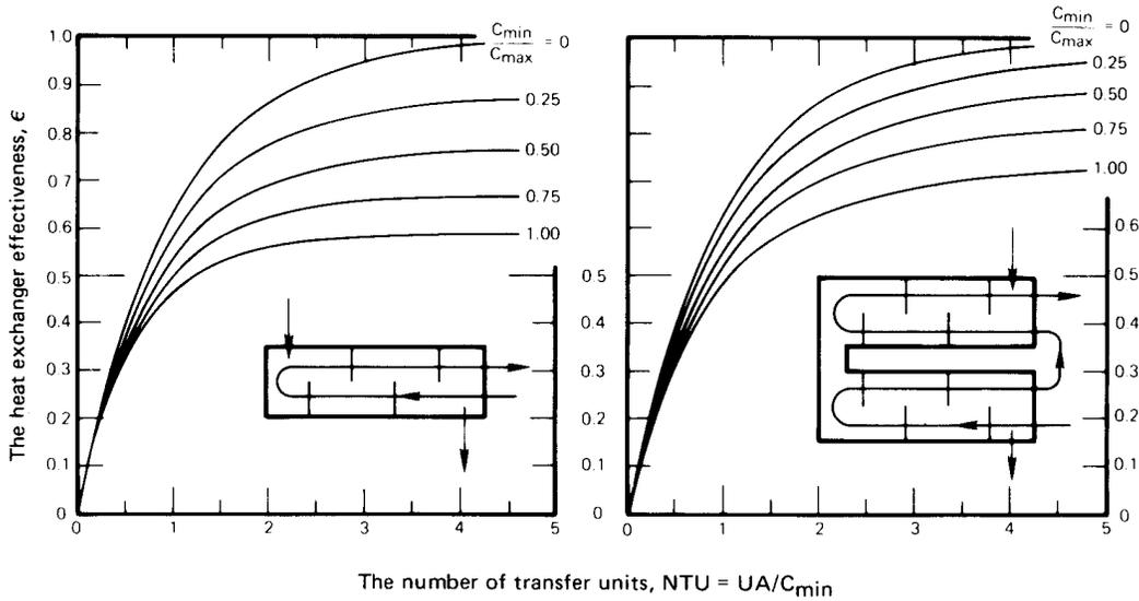
c.) One shell pass, two tube pass exchanger.
