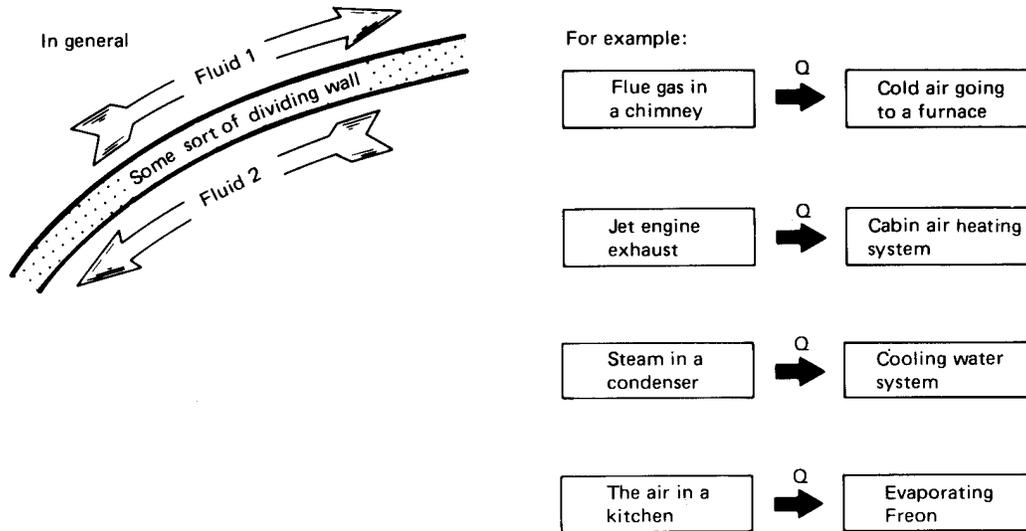
Figure 3.1 Heat exchange.
