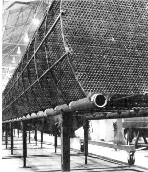
*Above and left:* A very large feed-water preheater. Tubes are shown withdrawn from the shell on the left. Inset above shows baffles before tubes are inserted. (Photos courtesy of Southwest Engineering Co., Subsidiary of Cronus Industries, Inc., Los Angeles, Calif.)
