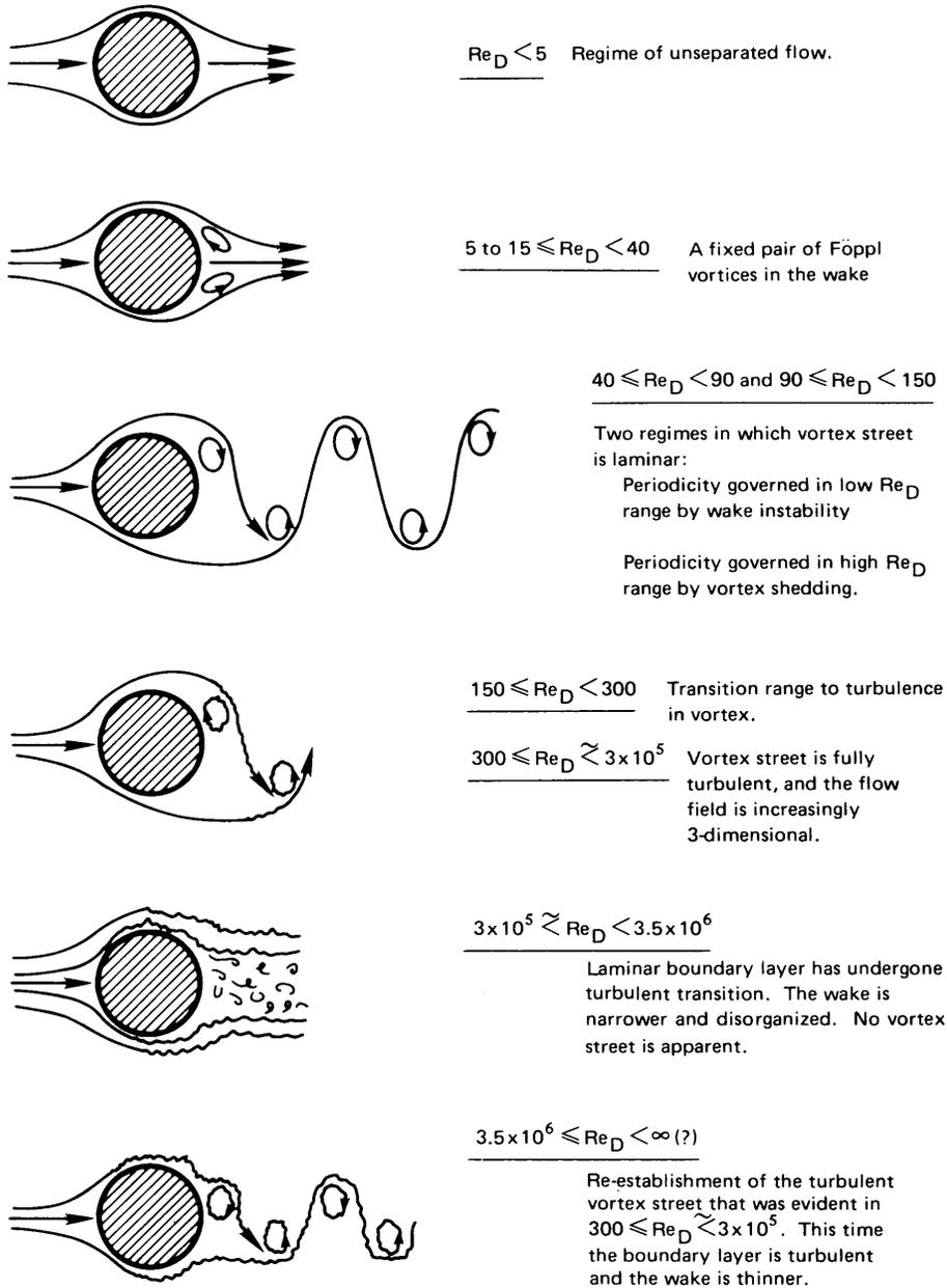
Figure 7.10 Regimes of fluid flow across circular cylinders [7.22].
