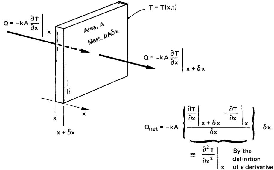
**Figure 1.8** One-dimensional heat conduction through a differential element.
