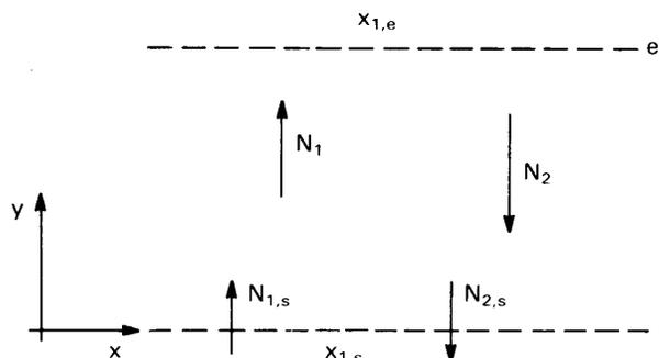
**Figure 11.16** Mass flow across a one-dimensional layer.
