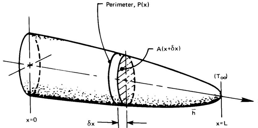
Figure 4.11 A general fin of variable cross section.
