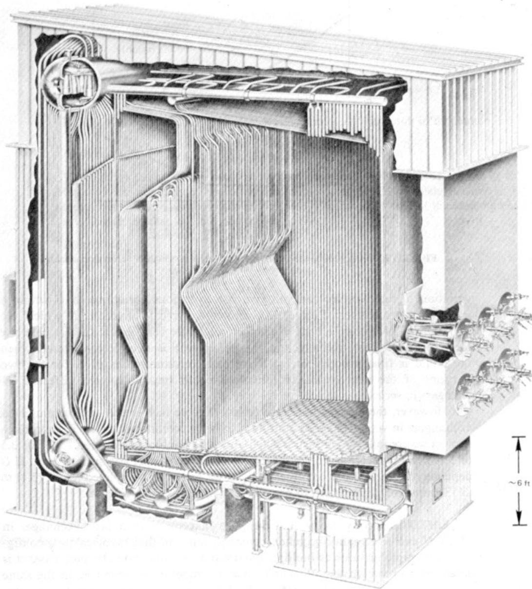
**Figure 3.12** The heat exchange surface for a steam generator. This PFT-type integral-furnace boiler, with a surface area of 4560 m<sup>2</sup>, is not particularly large. About 88% of the area is in the furnace tubing and 12% is in the boiler (Photograph courtesy of Babcock and Wilcox Co.)
