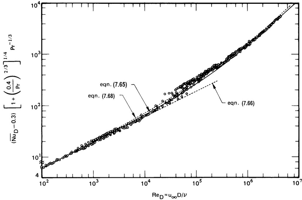
**Figure 7.13** Comparison of Churchill and Bernstein's correlation with data by many workers from several countries for heat transfer during cross flow over a cylinder. (See [7.24] for data sources.) Fluids include air, water, and sodium, with both  $q_w$  and  $T_w$  constant.
