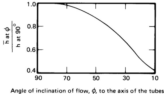
**Figure 7.16** Correction for the heat transfer coefficient in flows that are not perfectly perpendicular to heat exchanger tubes [7.26].
