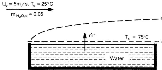
Figure 11.19 Evaporation from a tray of water.
