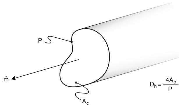
Figure 7.9 Flow in a noncircular duct.
