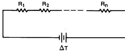
**Figure 2.18** A thermal circuit with many resistances.
