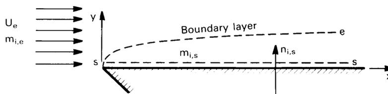
Figure 11.14 Concentration boundary layer on a flat plate.
